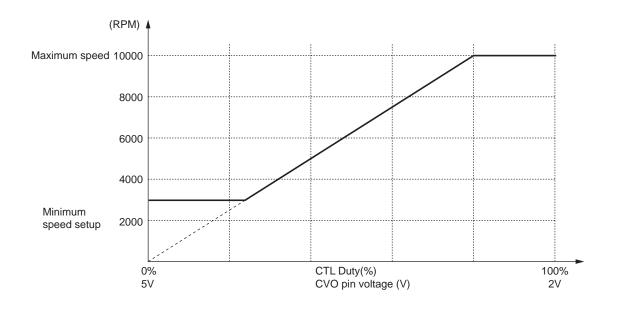
Obtain the ratio of the minimum speed required to the maximum speed. Ra = Minimum/maximum speed ··· (1) In the example shown in the figure above : Ra = minimum/maximum speed = 3000/10000 = 0.3
