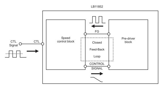
The operation inside the IC is as flows. pulse signals are created from the edges of the FG signals as shown in the figure below, and using these signals as a reference, waveforms with a pulse width determined by the CR time constant are generated using a one-shot multivibrator. These pulse waveforms are then integrated to control the duty ratio of the pre-driver output as the control voltage.
